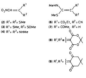
presence of a zeolite catalyst  $\dagger$  to give 1-methylamino-1-methylthio-2-nitroethylene<sup>6</sup> (1) (50%). The main advantages of this reaction are: (i) the catalyst can be recovered and re-used; (ii) the product is not contaminated with the unwanted 1,1-bismethylaimno-2-nitroethylene (4); (iii) the crude product obtained is >99% pure by GC and HPLC.<sup>‡</sup>
